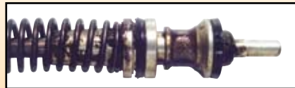
Harmful deposits and varnish build-up—resulting from worn-out, oxidized brake fluid—are apparent on this brake master cylinder piston assembly.
