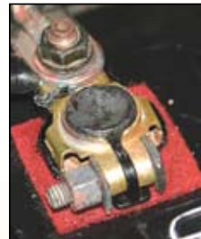
Battery terminal after BG Battery Service.
