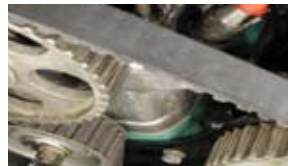
New Installed Timing belt
