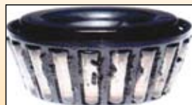
Heavy deposits reduce equipment life.
