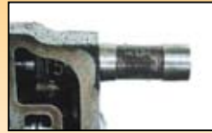
Valve body spool with heavy deposit build-up.
