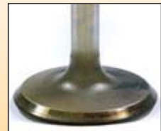
Intake after valve service.
