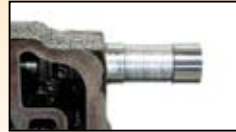
Valve body spool after BG Transmission service.
